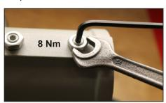
18. Losen two allen srews to set an angle of the luminaire. Tightening torque of 8 Nm.
