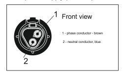
2. Connect the 3 core cable to the power supply (Class I.).
