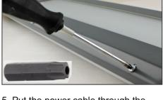
2. Unscrew the top cover using a Torx -
