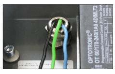
7. Connect the cable to the terminal block.
