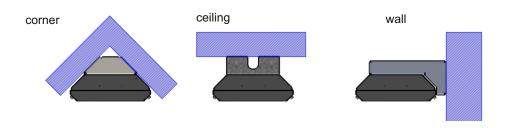
3. Drill two holes at the mounting location (ceiling/wall) - spacing according to the variant.
