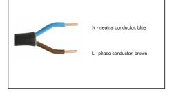
2. Prepare the luminaire for the instalation.
