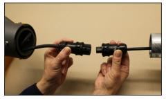
5. Connect the 3 pin connector Gesis to the power supply (Class I.).
