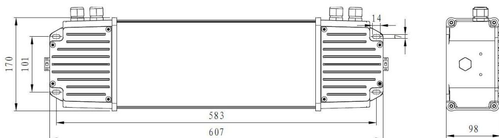
Dimensional diagram of the power supply box for NITRON 3
